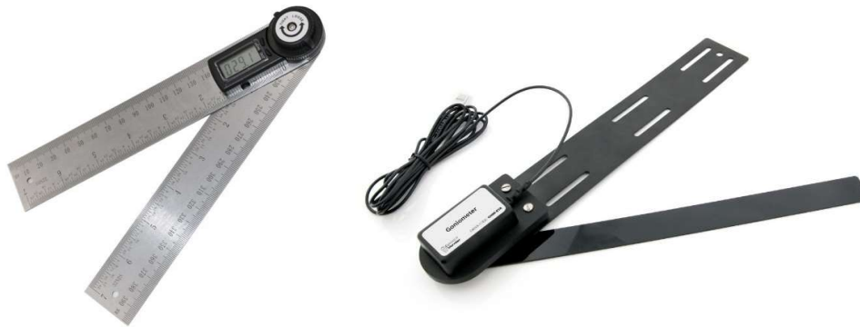
Figure 14: Measurement of the angle between thigh and calf with a digital non-connected goniometer and with a connected goniometer.
