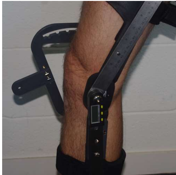
Figure 15: Measurement of the angle between thigh and calf with a digital non-connected goniometer attached to the brace.
