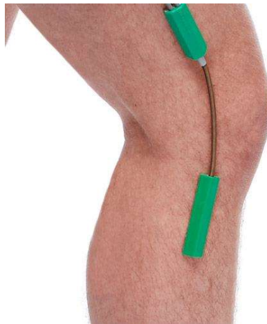
Figure 16: Flexible system to measure angle between the thigh and the calf with wireless data collection ( http://www.biometricsltd.com/goniometer.htm ).
