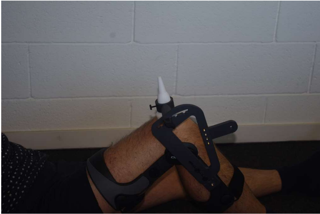
Figure 12: Actual brace with a probe positioned for imaging the patellar pole in the sagittal plane.
